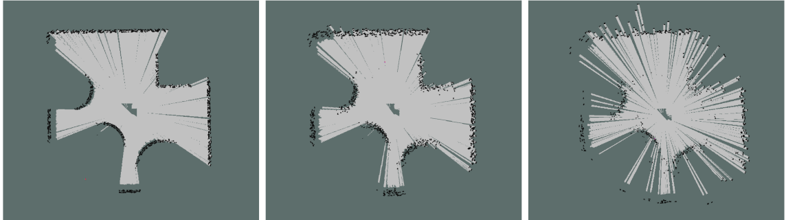
Figure 9.6: Comparison of maps generated using ground truth (left), LSTM+EKF (middle), and EKF-only odometry (right)
