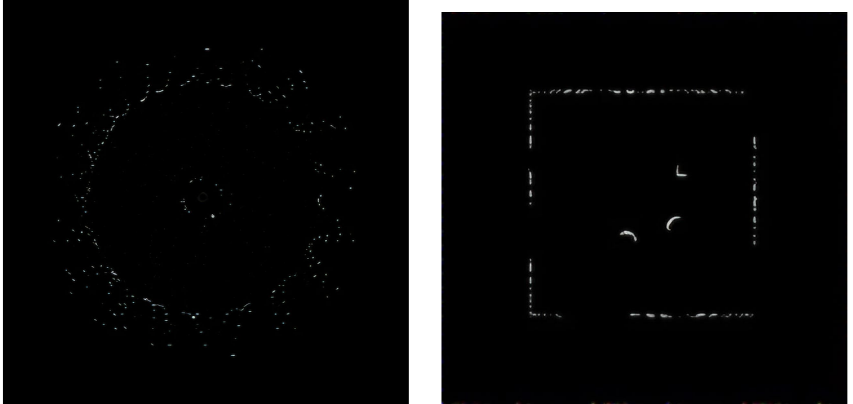
Figure 8.2: Motion Compensation: Distorted uncompensated sonar image (left) and Compensated Sonar Image(right)
